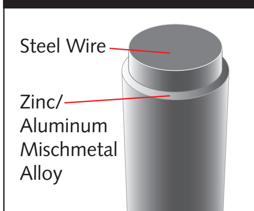
Cross-sectional View of CONZINAL
